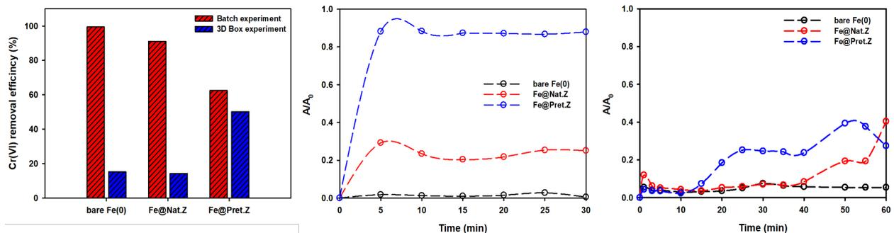
Fig.2 (a) Comparison result of Cr(VI) removal efficiency for each materials (bare Fe(0), Fe@Nat.Z and Fe@Pret.Z) in batch and 3D box experiment. (b) Column mobility test and (c) box mobility test results
