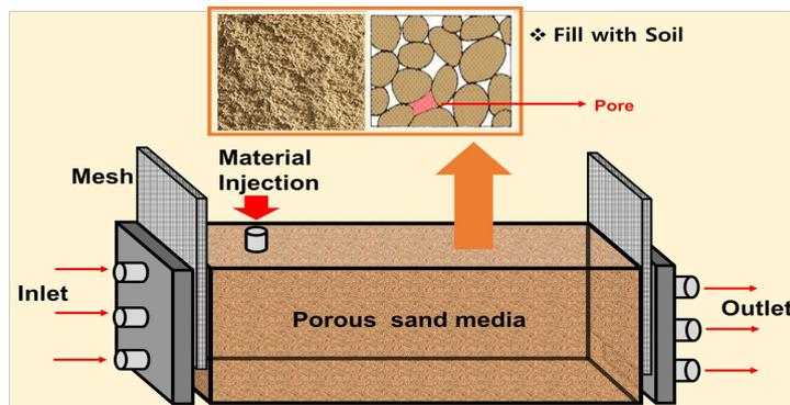
Fig.1 Designed 3D box type reactor
